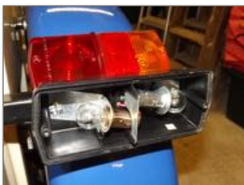
Lucas light fitting internal arrangement
