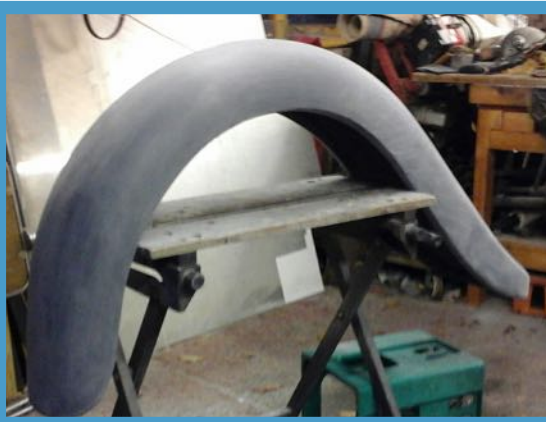
Above, getting the exact shape and return edges. Which will give the finished wings a lot more strength.
