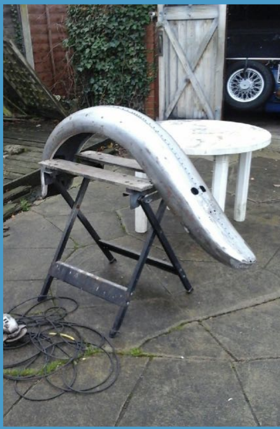
Above, getting the exact shape and return edges. Which will give the finished wings a lot more strength.
