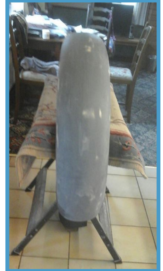
Filled and smoothed, this is the last stage before I take a mould.
