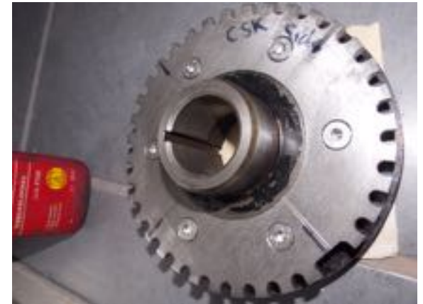
Trigger wheel with missing tooth at 5 o' Clock
