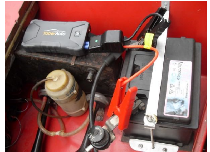
A small battery will suffice if helped by a booster pack. Usually cheaper than a bigger battery, just needs a little camouflage.
